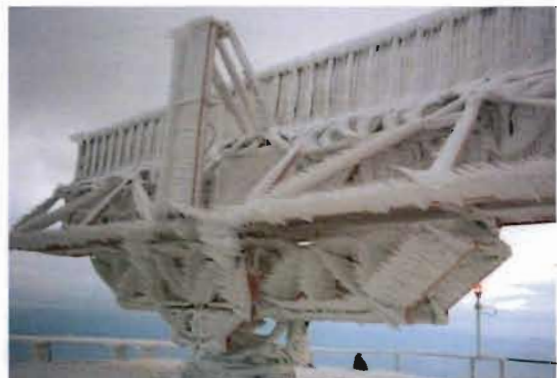
Figure 1 - A picture of the antenna ALE9 operating on a site exposed to severe outdoor requirements
